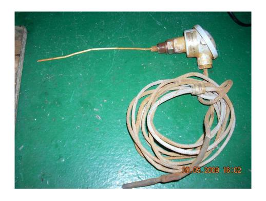
Damaged temperature sensor
